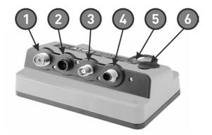
To avoid damage to the cables, ensure at least 50mm (2.0 inches) is available below the Transceiver to allow the cables to turn.
