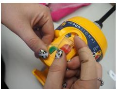
The cover should now lie flush to the surface if all is well. To slide the red key back to the off position, open up a paper clip and poke it into the small hole in the bottom of the cover and push upwards. The clip should now be in place.
