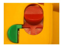
Offer up the clear cover, locating the round lug at the bottom first. With the clip at a slight angle (anticlockwise from the top), press the clip at the bottom into the oval recess. This is the tricky bit and takes a little trial and error! The only problem is an error usually breaks the clip.
