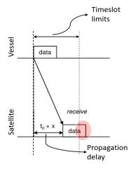
The figure shows a red area where the data will collide with the next timeslot. When compressing the data, the transmission will fall between the boundaries set for a timeslot. This will improve the reliability for reception by AIS satellites.
