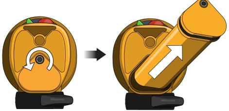
Insert new battery pack, ensuring that the rubber seal is correctly in position.
