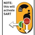
∆ Whilst holding the red switch down, release the areen switch to lock in active position.
