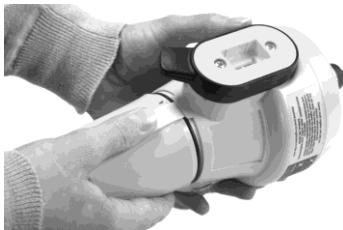
3. Push the battery home and **lightly** tighten the bolt with the supplied Hex (Allen)
